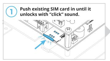
Remove existing SIM card and locate new SIM card.
